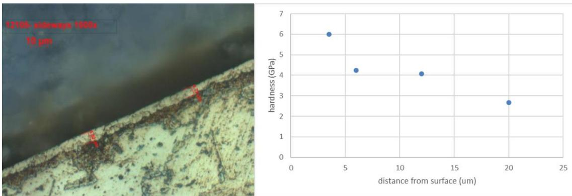
Figure 6 metallographic section and hardness profile for steel 1215 grade nitride at Duralar with a 1h process at 500 °C
