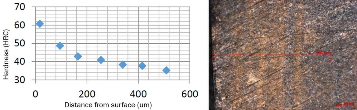
Figure 5 4140 steel - hardness profile and sectioned sample for a HC nitriding process performed at Duralar
