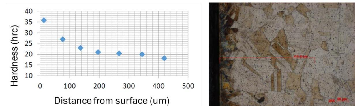
Figure 1: AISI 316L - hardness profile and sectioned sample for a HC nitriding process performed at Duralar
