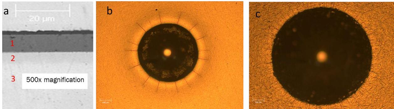
Figure 10 metallographic section and VDI indent of a duplex coating (10m DLC on the top of a 8 $\mu\text{m}$  thick nitride layer). Panel a) metallographic section of the sample. 1 is the coating, 2 is the nitride compound layer, 3 is the diffusion area. Panel b) VDI indent on the coating on a A2 tool steel sample; panel c) VDI indent of the coating on a 316L stainless steel sample
