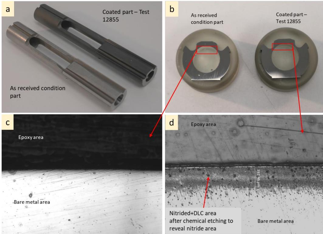
Figure 11: bolt carrier as-is and after duplex (nitriding+dlc) coating. The figure reports the status in 4 panels, depicting the bolt carriers as-is and coated (panel a), the cross section (panel b), and the micrographs (panels c and d)
