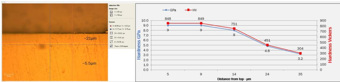
Figure 3 – metallographic section and hardness profile for a 20μm nitride layer
