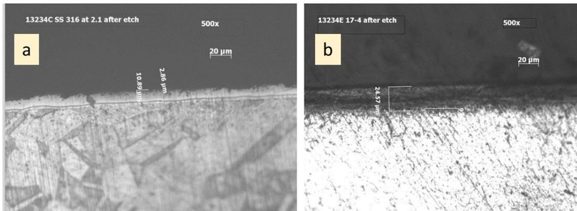
Figure 8 1h nitride process at 440 °C on 316L (panel a) and 17-4 (panel b)
