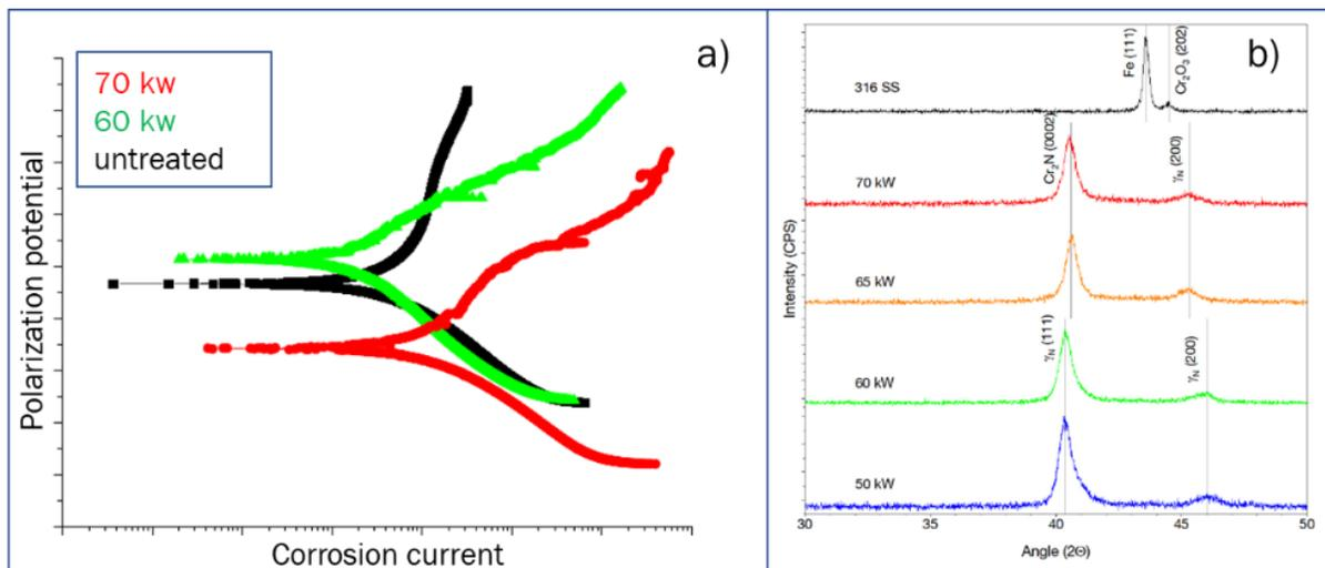
Figure 2 – panel a) Tafel plot for AISI 316 in HC plasma for 60 minutes at 60kw and 70 kw; panel b) XRD spectra of untreated and samples nitride at 50, 60, 65 and 70 kw
