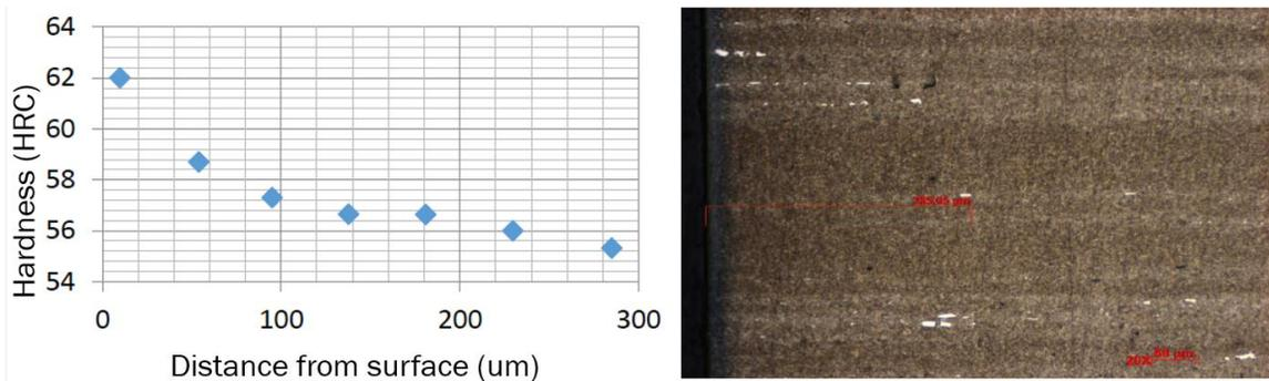
Figure 4 : D2 Tool steel- hardness profile and sectioned sample for a HC nitriding process performed at Duralar
