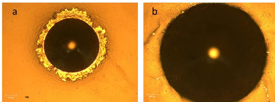
Figure 9: VDI indentation of 10 um coating deposited on A2 tool steel coupon (panel a) and 316 L stainless steel (panel b)
