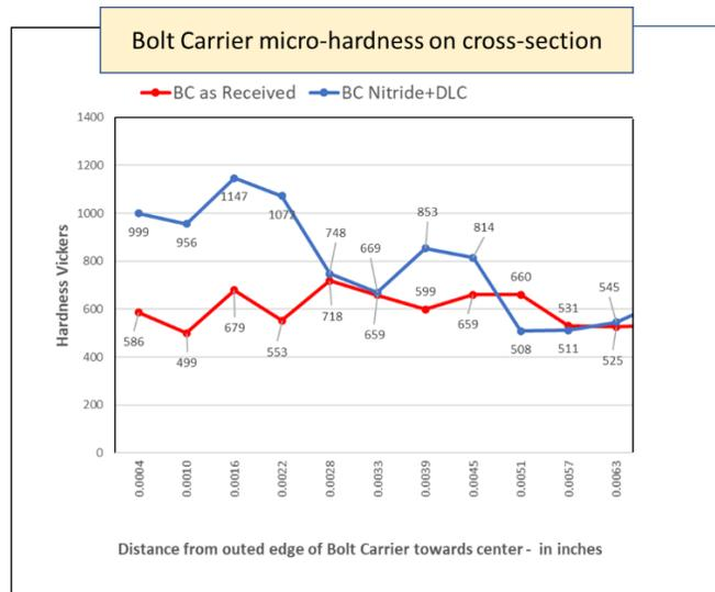
Figure 12: microhardness of the bolt carrier cross-section as a function of the distance from the substrate surface
